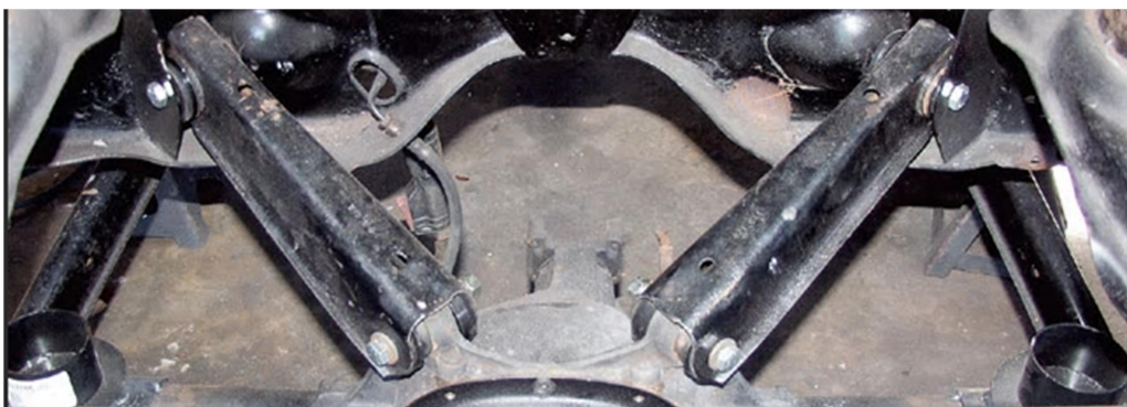
The metric 4 link rear suspension (OEM stock looking from rear to front)
